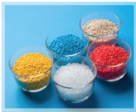
NORYL : NORYL resins offer a good balance of mechanical and chemical properties . very low are the level of water absorption and thermal dilation , therefore it is most suitable in thermo – hydraulical field , not containing lead and maintaining a long – term electrical insulation capability and thermal resistance.
